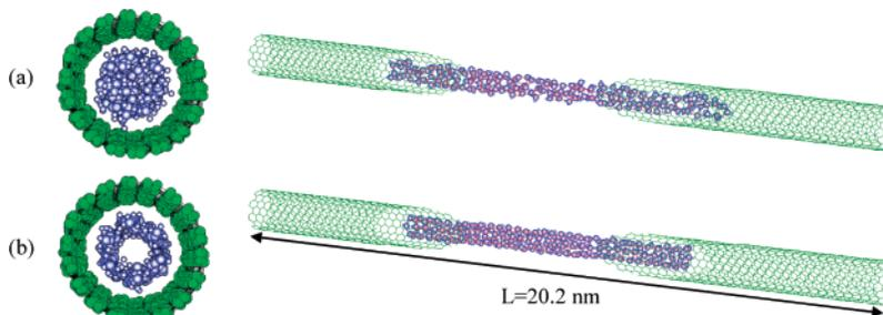
**Figure 1.** (a) Typical initial condition of a saturated water cluster in a (9, 9) SWNT and (b) the ice-nanotube crystallized by cooling the SWNT to 200 K ( $n = 6$ ).
