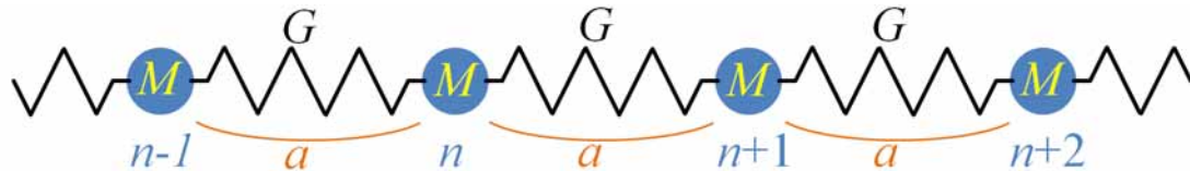
Fig. 1-1 One dimensional harmonic oscillator model: one atom in a unit cell.
