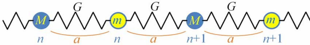
Fig. 1-2 One dimensional harmonic oscillator model: two atoms in a unit cell.
